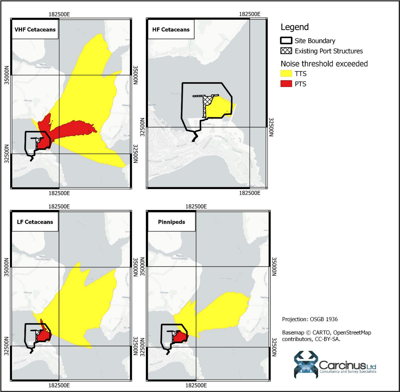
Figure 9.18 Noise threshold exceedance for different marine mammal groups as a result of demolition of the Northern Arm.
